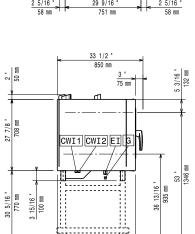
C- = Cold W WI- (cleaning) Cold Water inlet 1
